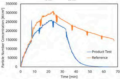
Particle Number concentration measured over time. The smoke phase occurs during the initial 25 minutes, which is followed by a 10-minute mixing period. Hereafter the air purifier is turned on (only for product test) for 30 minutes.
