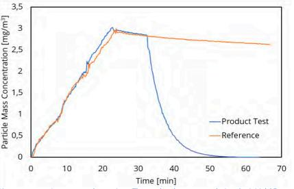
Particle Mass concentration measured over time. The smoke phase occurs during the initial 25 minutes, which is followed by a 10-minute mixing period. Hereafter the air purififer is turned on (only for product test) for 30 minutes.
